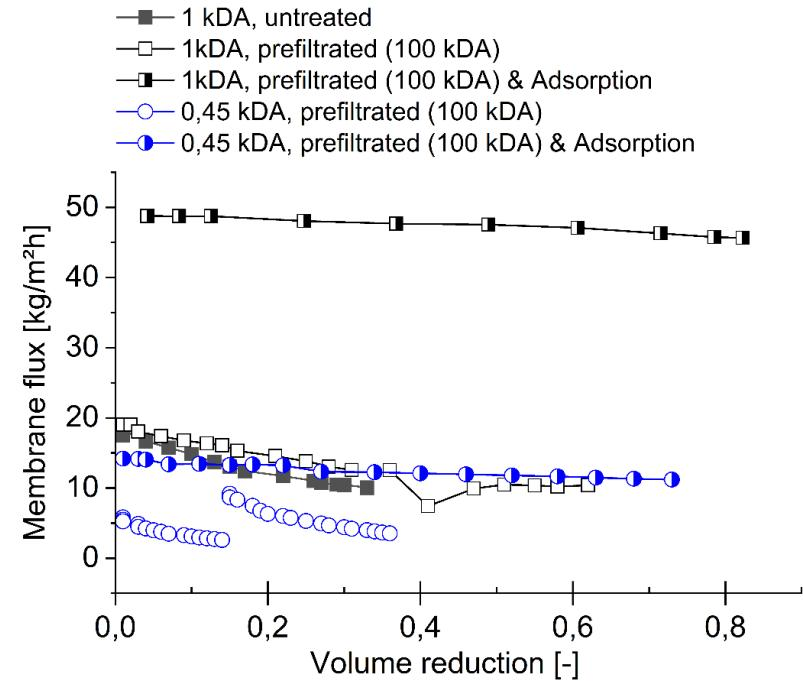
All experiments were conducted under the same operation conditions: Temperature: 40 °C / Transmembrane pressure: 4 bar / Cross flow velocity: 2.3 m/s
